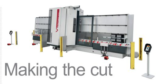
(patented by Intermac) reduces manual handling and keeps the glass in the vertical plane, from rack to machine. The pieces can be either multiples of the same piece, or 'batch one' (single items), so the benefit of zero setup means time savings over traditional flatbed CNCs, including the Master series, and can save up to 30% in time.
